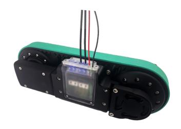
The Track Actuator is a full-featured robotic component as opposed to a simple servo motor. The output rotates continuously, requires no calibration or homing on boot-up, and wiring can be easily daisy-chained. This configuration enables the actuators to be a versatile tool for mobile robotics platforms.
