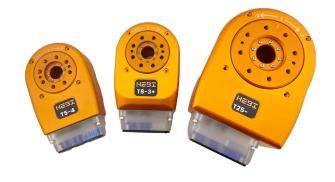
The T-Series Actuator® is designed to function as a full-featured robotic component as opposed to a simple servo motor. The output rotates continuously, requires no calibration or homing on boot-up, and contains a thru-bore for easy daisy-chaining and wiring. This feature enables these actuators to be used in everything from wheeled robots to multidegree of freedom collaborative robotic arms.
