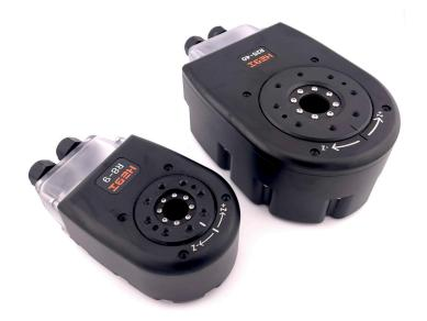
The R-Series Actuator is a full-featured robotic component as opposed to a simple servo motor. The output rotates continuously, requires no calibration or homing on boot-up, and contains a thru-bore for easy daisy-chaining of wiring. This enables the actuators to be used in everything from wheeled robots to collaborative robotic arms.
